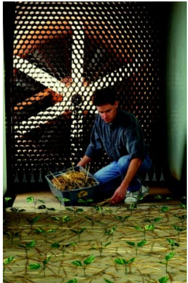
Figure 3.2. In a wind tunnel, a technician prepares to measure how live plants and straw residue slow windblown soil erosion. Photo by Scott Bauer, Agricultural Research Service, U.S. Department of Agriculture, Beltsville, Maryland.
