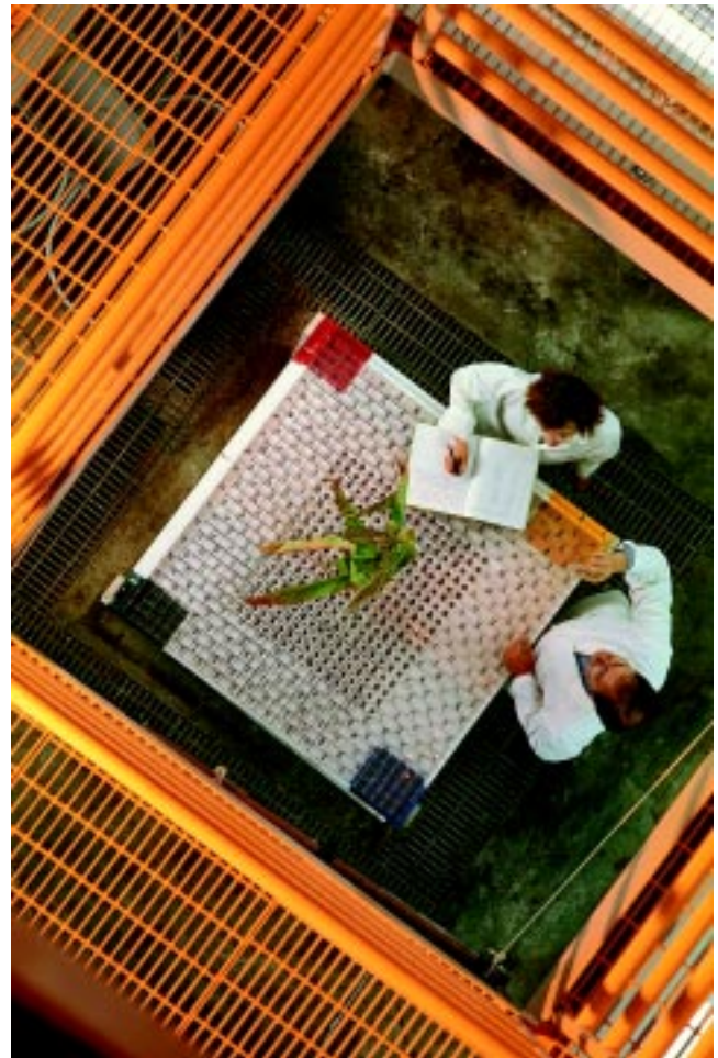
Figure 3.3. Technicians at the base of a 3-story rainfall simulator study rainfall interception by foliage. Photo by Scott Bauer, Agricultural Research Service, U.S. Department of Agriculture, Beltsville, Maryland.
