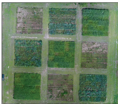
Figure 5. UAV-collected aerial survey of bioenergy crops in Williamsdale, North Carolina (left) and UAV-derived three-dimensional surface model of various bioenergy crops. In-season biomass is estimated using the remotely measured canopy heights. Photos from R. Austin and C. Crozier, N.C. State University.
