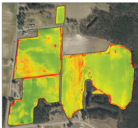
Figure 4. Vegetative health of sweet potato fields as measured from UAV-based imagery one week before harvest (left). A strong spatial correlation exists with soil color as observed in the image on the right. Photos from R. Austin N.C. State University.
