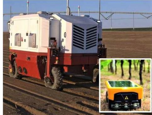
A Seattle-based robotics company's "autonomous weeder" [uses lasers to kill weeds](#). And French researchers have used cues from Mars rovers to develop [a weed robot for the vineyards](#).
